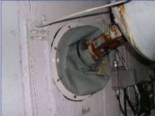
Figure 120.5 CB Boot Installation Complete
