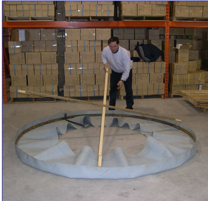
Figure 130.5 96" – 98" Pipe to Pipe Boot Size Verification
