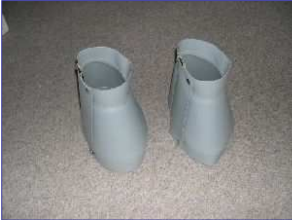
Figure 130.1 Pipe to Pipe Boots. Finished Product.
