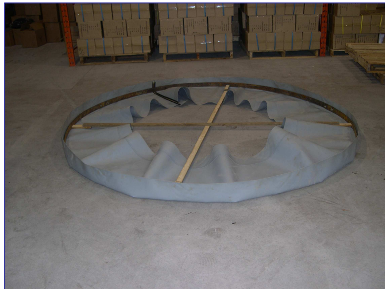
Figure 130.6 96" – 98" Pipe to Pipe Boot Size Verification
